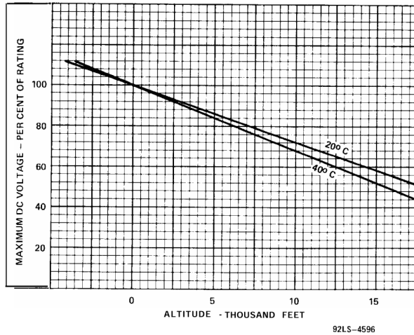
Figure 1 - Maximum DC Voltage with Respect to Altitude Forced Air Cooling
