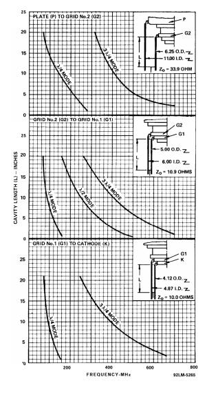
**Figure 5 - Typical Constant Current Characteristics**
