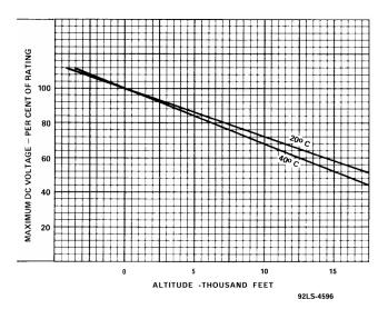
Figure 1 - Maximum DC Voltage with Respect to Altitude
