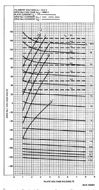
Figure 4 - Typical Constant Current Characteristics
