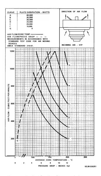
Figure 3 - Typical Cooling Characteristics
