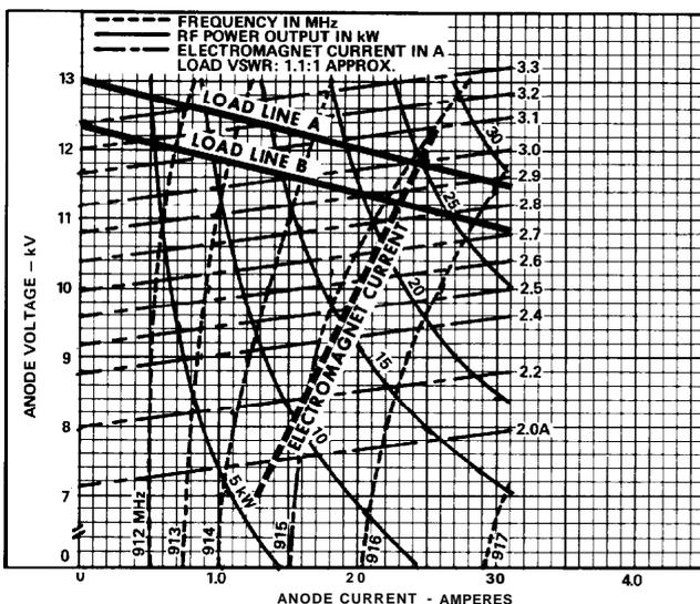
Figure 2- Performance Characteristics with Series-Excited Electromagnet
