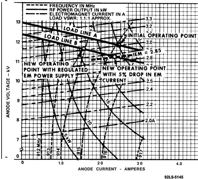
Figure 1 - Performance Characteristics with Separately-Excited Electromagnet
