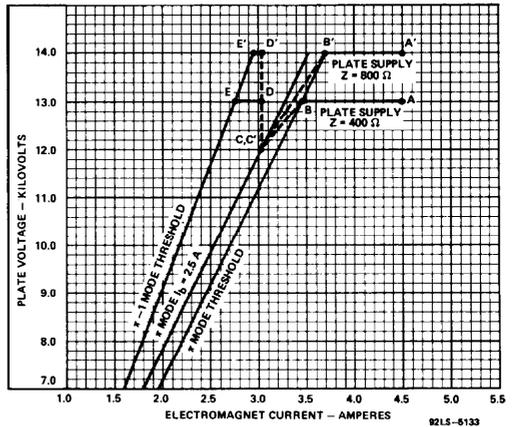
Figure 3 - RF Mode Characteristics
