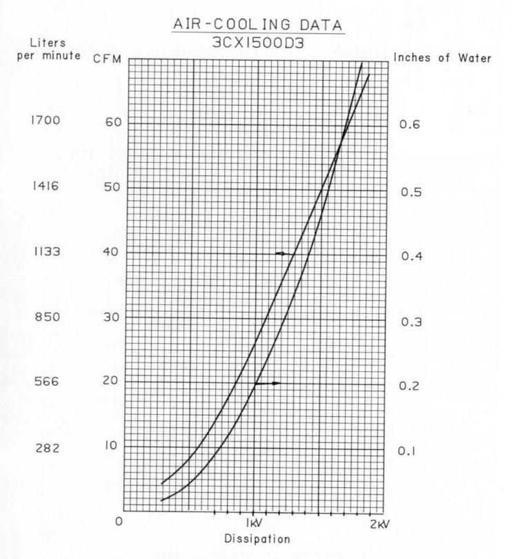
CFM and pressure required to keep anode temperature at 225°C.
