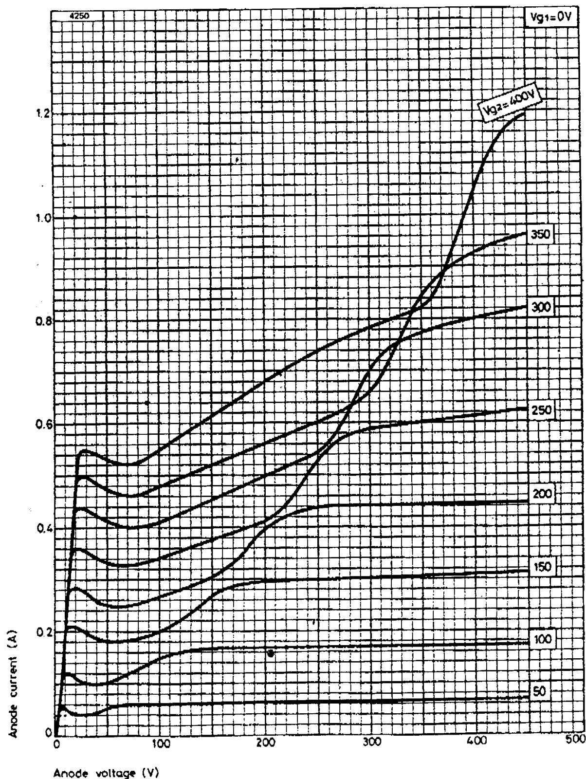
**SCREEN CURRENT-ANODE VOLTAGE AT  $V_{g1} = 0V$  WITH  $V_{g2}$  AS PARAMETER**
