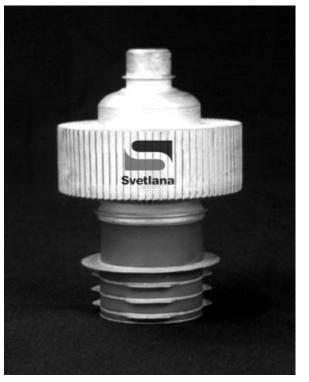
The Svetlana 4CX1500A is a high-performance ceramic/metal, forced air-cooled, power tetrode designed for use in Class AB<sub>1</sub> or Class C RF amplifier service. It may also be used for audio frequency modulator, pulse modulator and DC power regulator service. The 4CX1500A filament is precision fabricated in a cylindrical mesh configuration for exceptional mechanical stability and long life.
