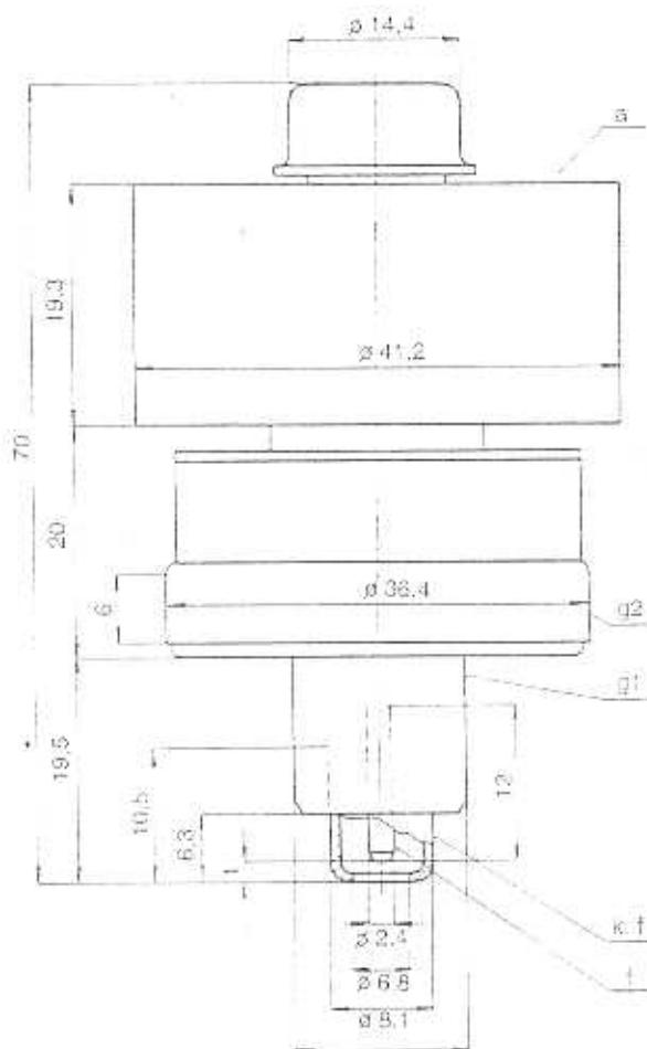
The RE 025 XM is a forced-air cooled, ceramic/metal tetrode for frequencies up to 1000 MHz, with coaxial arrangement of electrode terminals.
