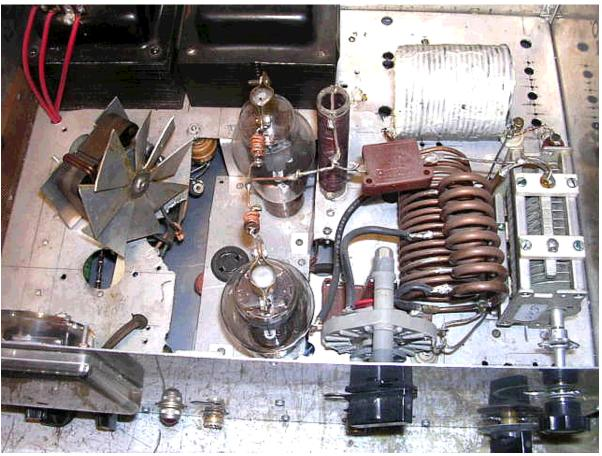
the cap loose, two very beefy power transformers (wired in series - possibly from TV sets, but no way to know), some decent quality variable caps, and other parts. But there is NO WAY this amp should be made to work in this condition and I am guaranteeing it to be DEAD ON ARRIVAL! The last thing I want is for the buyer to become dead instead!
